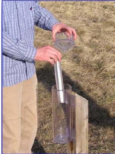
\* Warmer weather means it's time to place the inner cylinder and funnel back on your rain gauge. ***Remember to remove them, however, if freezing weather is in the forecast!***
